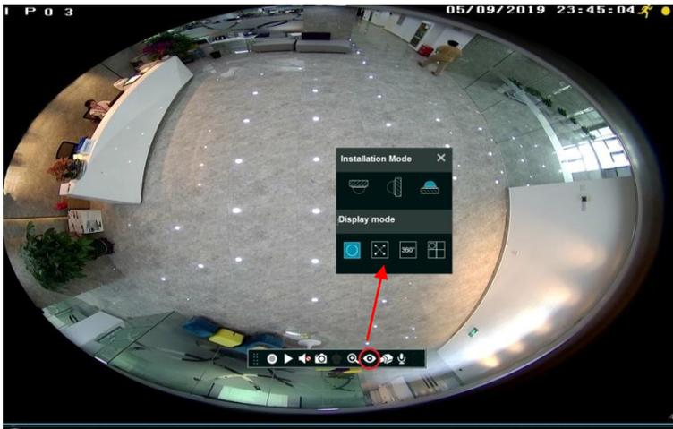
In addition, if this function is unavailable in the device, you can set the display mode and the installation mode via Web Client. To log in the web client, please refer to [Remote Surveillance](#)
